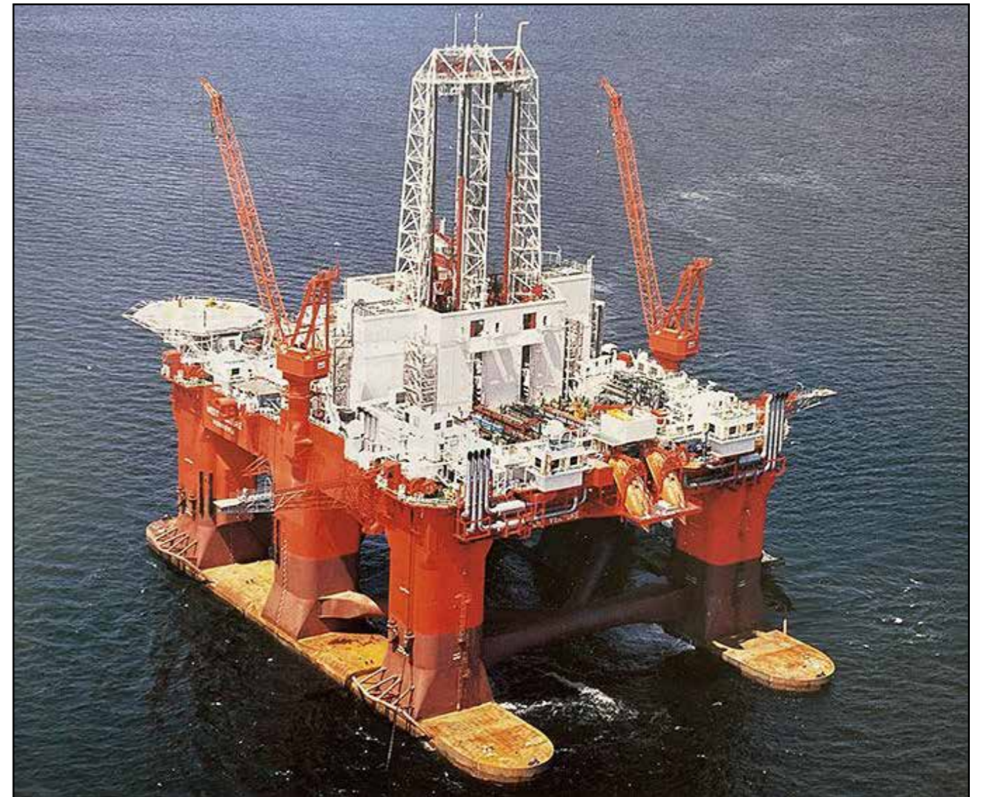
In September 1999, Hitachi Zosen completed the fifth-generation semisubmersible West Venture for Smedvig Offshore. It could operate in 1500 m water depths, with twin derricks permitting simultaneous drilling of two wells.
