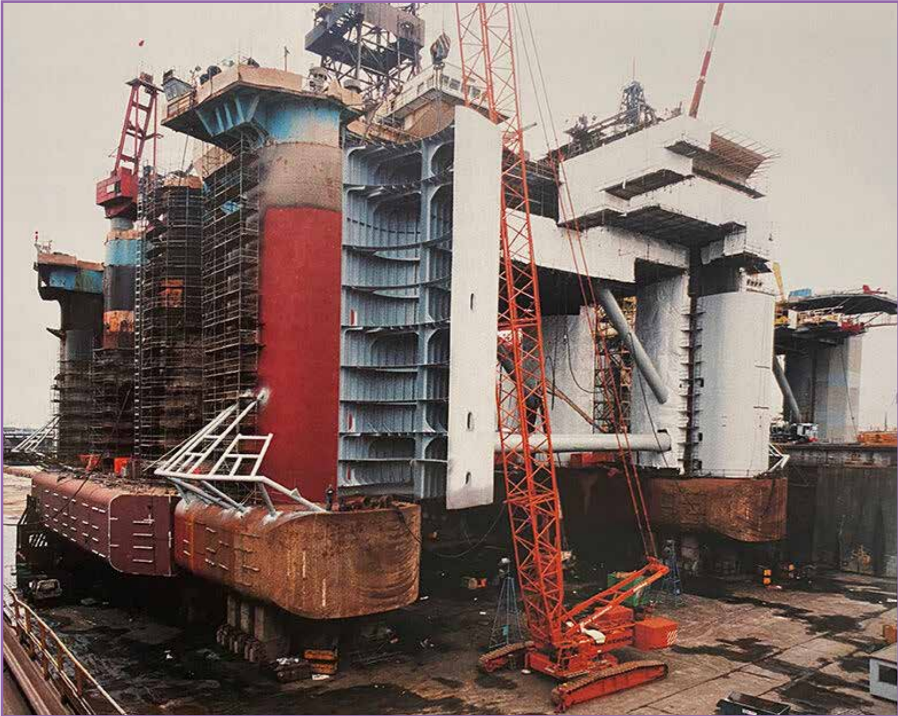
Global Marine Drilling purchased the Maersk Vinlander and drydocked her at the Verolme Botlek yard. Four blister tanks were added on the columns and two outer and inner sponsons added. It was renamed the Glomar Grand Banks
