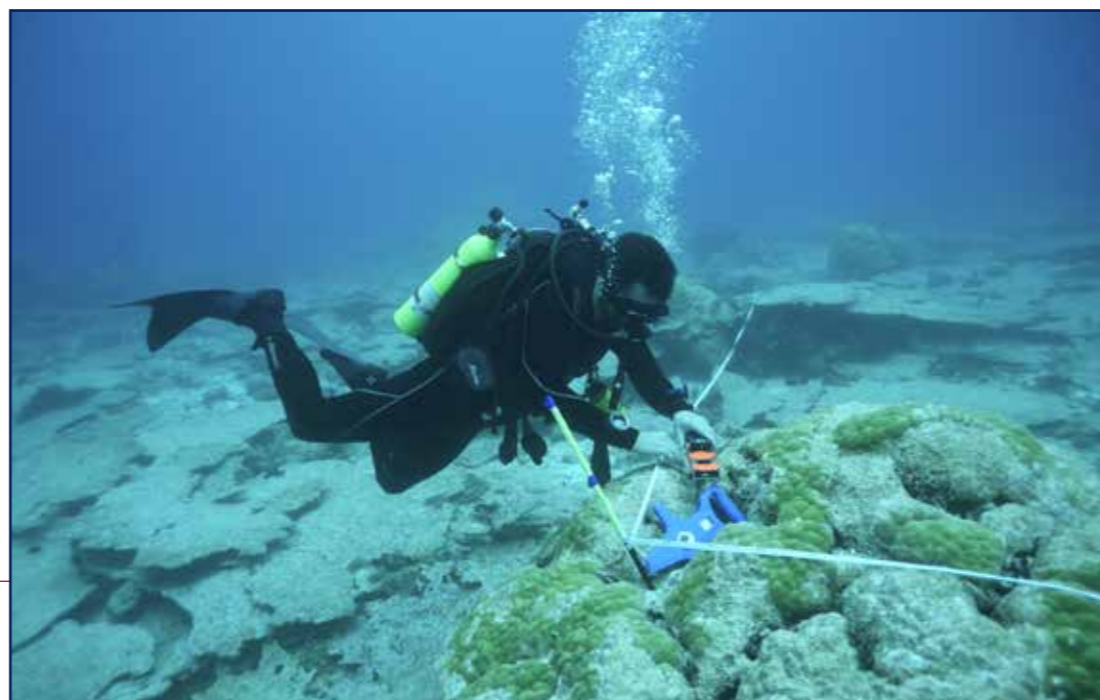
A diver setting up a temporary quadrat with scaling bars prior to collecting the photographs required to generate a 10 x 10 m 3D model of impacted coral in the Indian Ocean.
