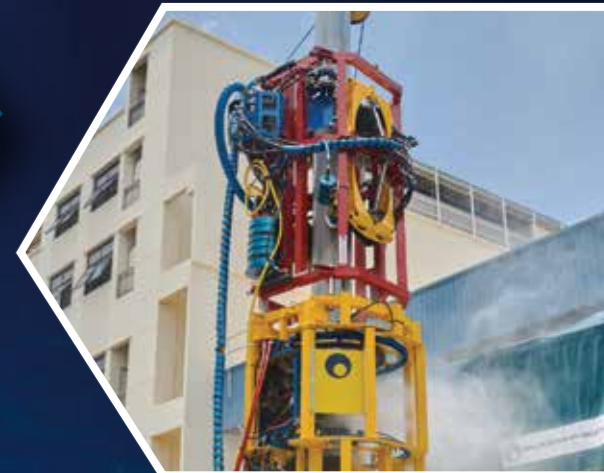
Roto Climber® Mk 2 on a pile with Traction unit on top and Cleaning, Close Visual Inspection and PAUT Module below.
