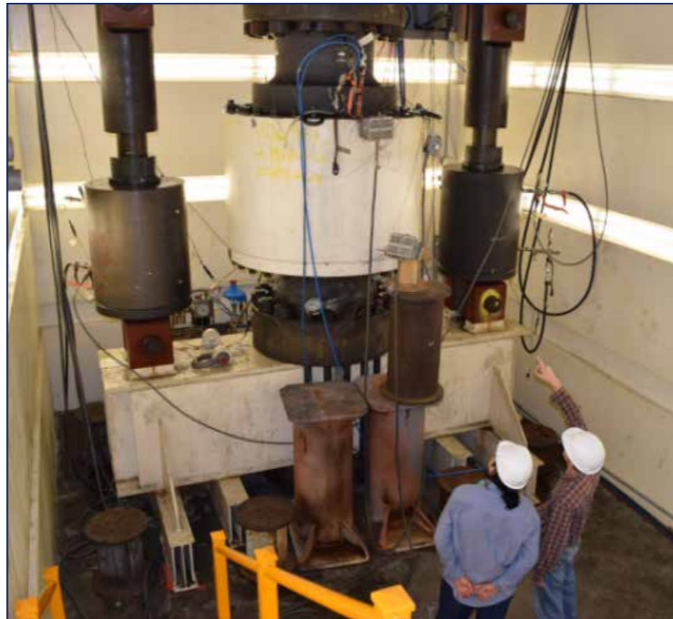
The connector was outfitted with strain and pressure gauges and tested at its full rated working pressure (20 ksi in the bore) with applied loads in bending, tension and compression. Image: Dril-Quip
