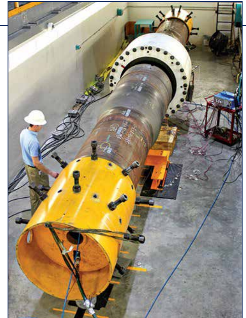
A complete 18 3/4-inch wellhead system with a DXe profile and wellhead connector was subjected to more than 90 million cycles, with an applied bending moment of 1,500,000 ft-lbf., over the course of four months of continuous testing. Image: Dril-Quip
