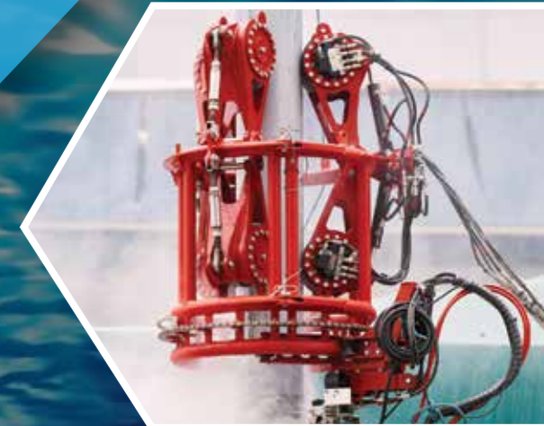
Roto Climber® Mk 1 on a pile. It is equipped with 2 each barracuda nozzles and a Cygnus WT Probe and video cameras.
