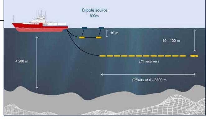
typically with a peak output current of 1.25kA, although source currents up to 7kA have been used.
