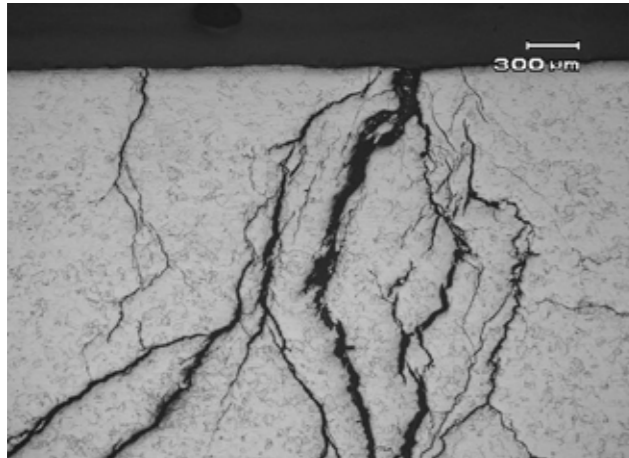
Stress corrosion cracking
