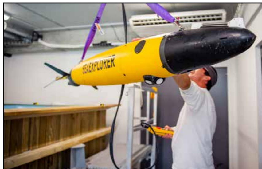
The Nortek ADCP’s small form and low profile enabled Alseamar to fit it to the SeaExplorer with little impact on the glider’s hydrodynamic properties
