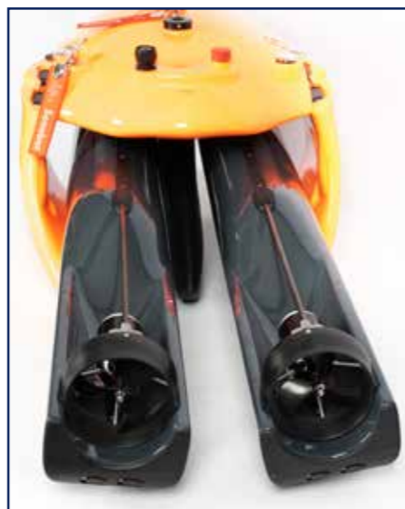
The Sonobot 5 is designed to be folded by hinges and secured quickly by latches instead of screw threads
