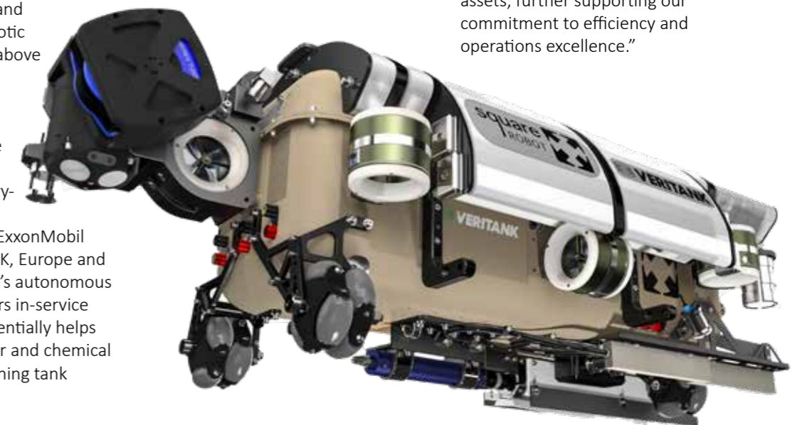
The Square Robot vehicle with the four-transducer Nortek DVL1000 mounted at the extreme left. The vehicle deploys ultrasonic testing, HD cameras and other non-destructive methods to assess tank wear and tear; the assessment depends on the DVL for pinpoint positioning.
