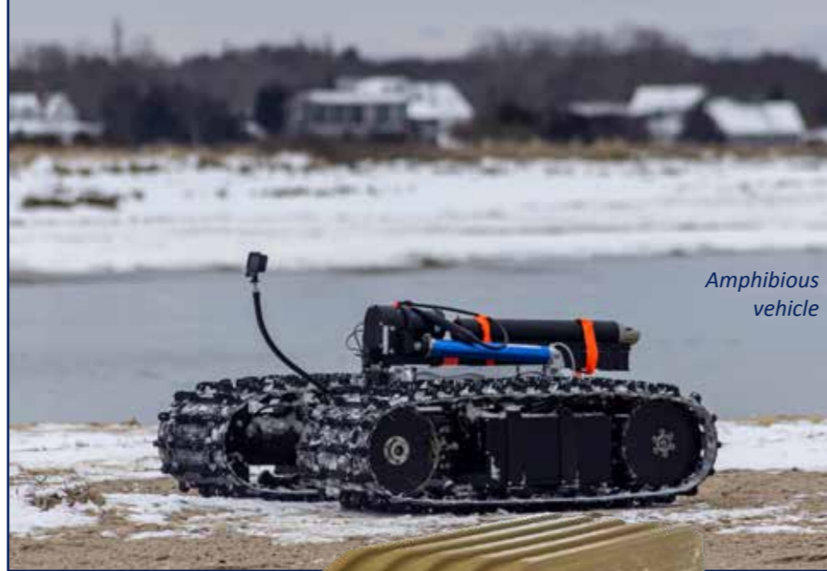
The Sea Beast, the largest amphibious crawler can carry 0.5t
