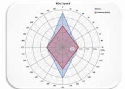
An ROV speed rose. The Isurus (blue) achieves a greater speed than traditional ROVs (red)
