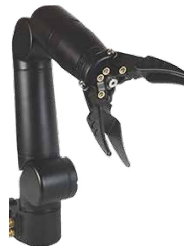
The Bravo 5 Five-function manipulator arm has a 0.67 reach where it can lift 12kg
