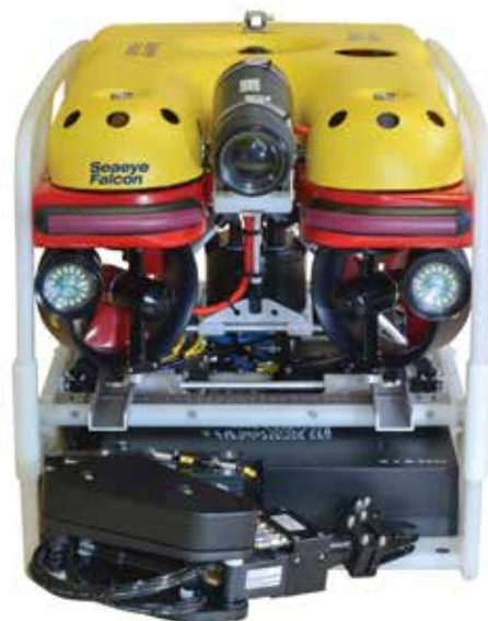
Falcon DR with five function manipulator skid
