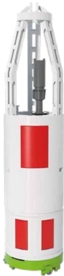
The smaller 2.820m dia OFD system produces a 3.140m dia hole. The drilling head turns at up to 14 rpm and the 400 kW drive produces a nominal torque of 708 kNm. The 13.5m machine weighs 100t
