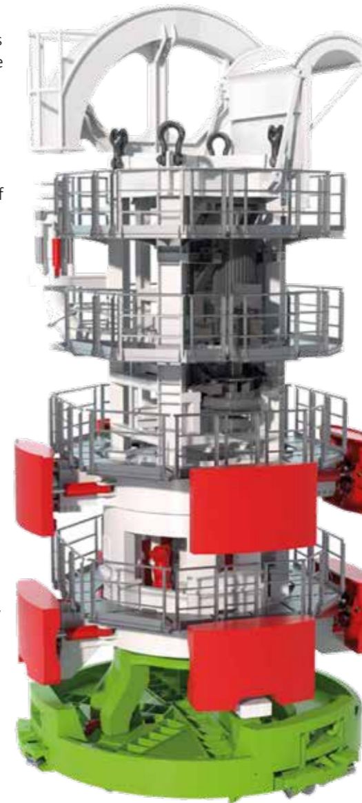
The larger 7.05m dia OFD system produces a 7.7m dia hole. The drilling head turns at up to 5.9 rpm and the 1600kW drive produces a nominal torque of 5,362 kNm. The 15m machine weighs 350
