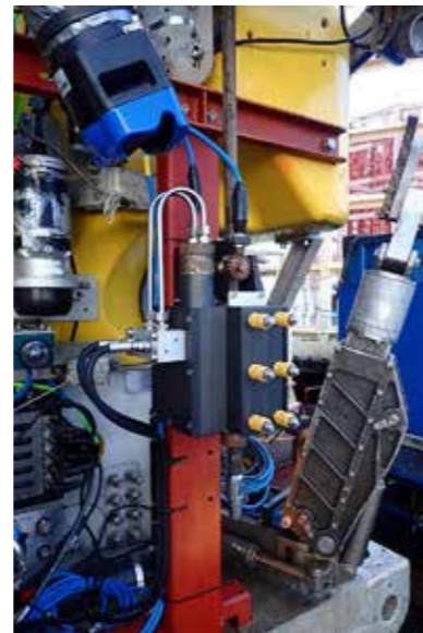
Bluefield Geoservices' ROVCone penetrometer and the ROV which eliminates cabling, reduces snag hazards, and speeds up installation and removal to/ from the ROV.
