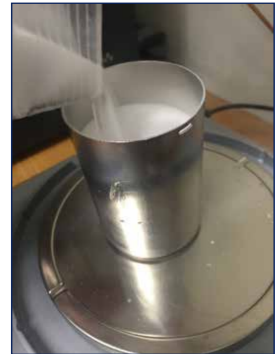
Eccospheres being weighted before testing
