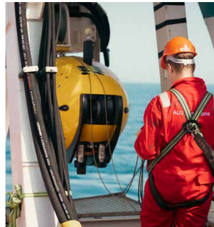
Nose section of the Autosub 5 Left: Preparing the Autosub for operations
