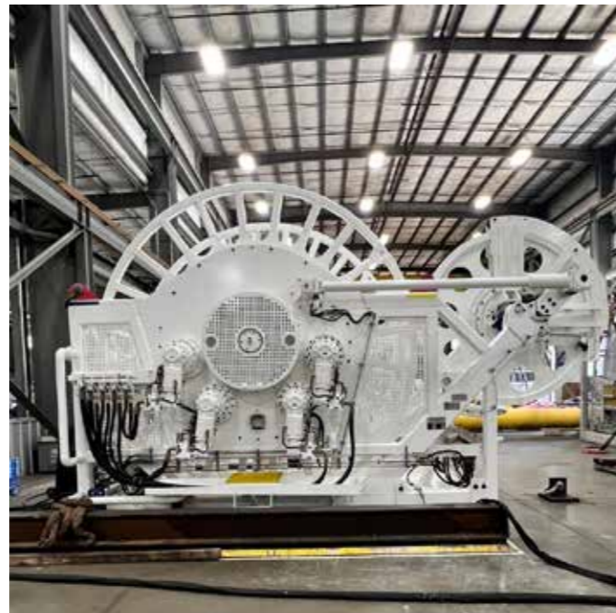
Logan Industries' coiled tubing (CT) reeler suite for OneSubsea,
