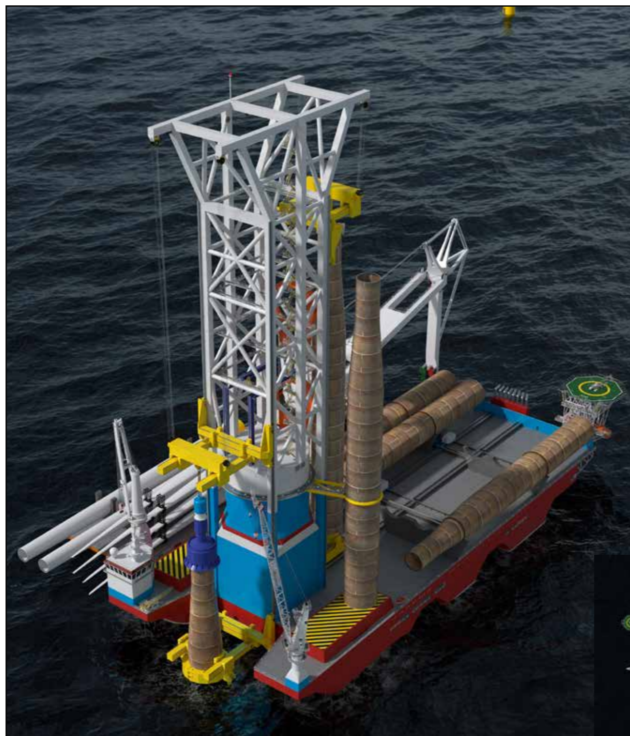
Installing a monopile
