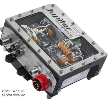
unit in-house for inspection and run it through our it environmental chambers for temperature cycling. It then goes for bench testing and ultimately pressure testing. This is done for every subsea PCB as standard before it is allowed to be
