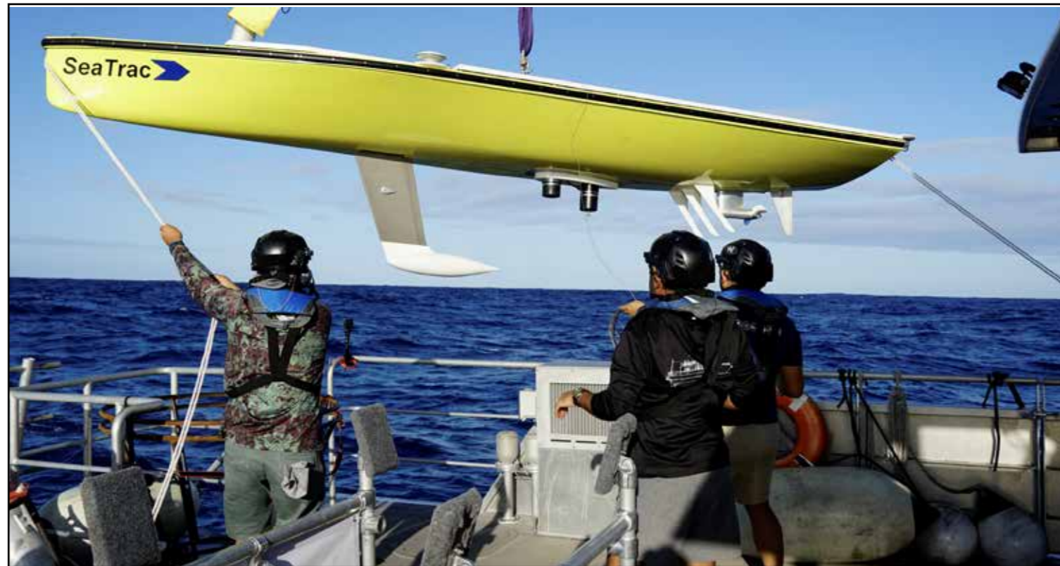
Above: It has four GPS receivers and two acoustic transducers (seen protruding from the hull just aft of amidships).
