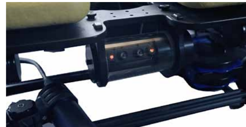
The camera can revolve to move up and down. Laser pointer can add a scale
