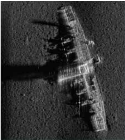
Sonar scan of the BV-222 fuselage captured using Hugin AUV. Photo: HUGIN Team 1 / Forsvaret
