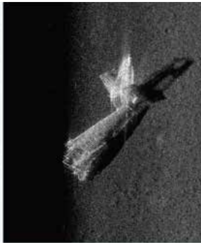
Sonar scan of the BV-222 tail section captured using Hugin AUV
