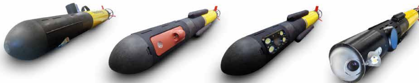
A single NemoSens can be configured with various payloads such as camera, lights, DVL, CTD sensor, SSS
