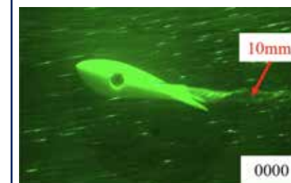
Flow change with the addition of tubercles
