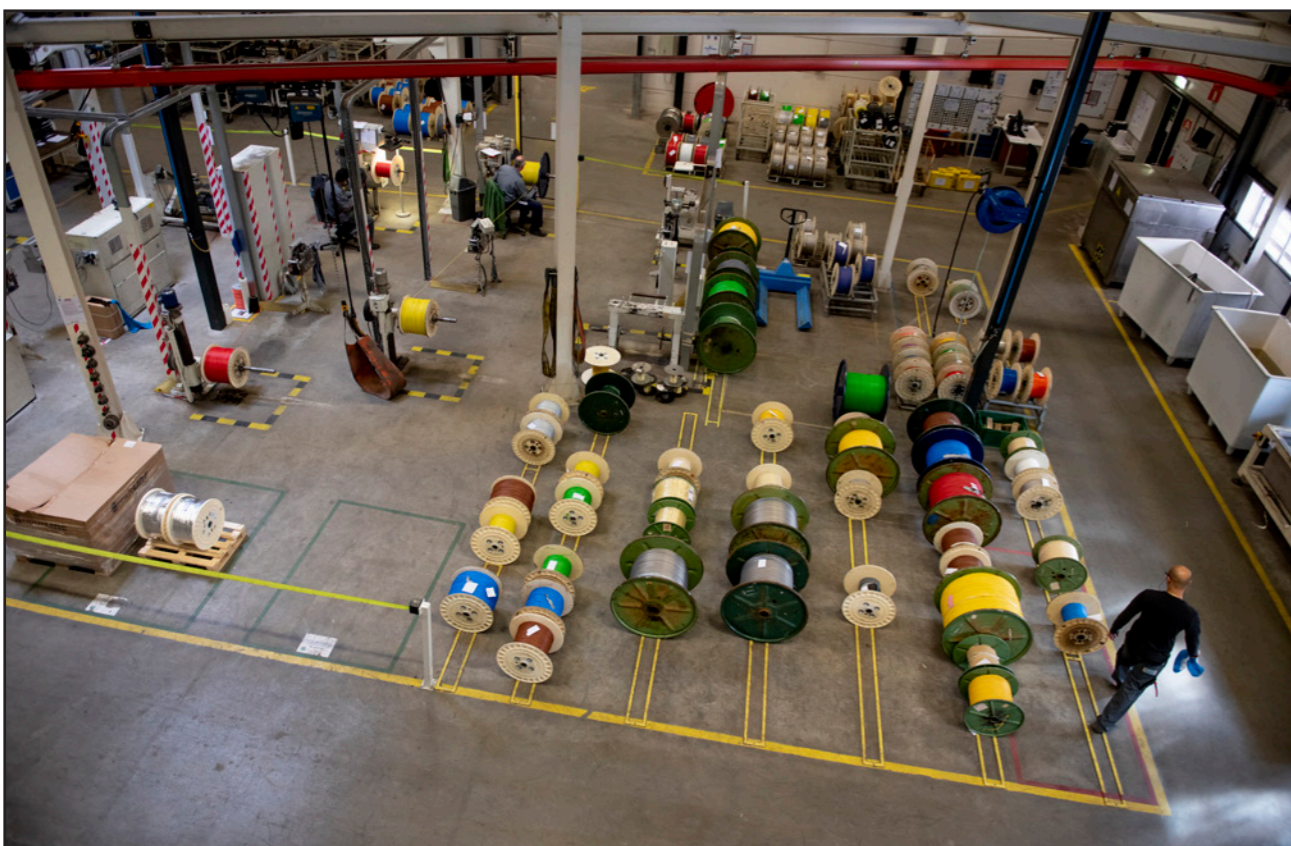
Stored bobbins containing individual cable subcomponents waiting to be installed on the lay up machine
