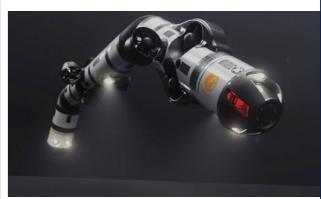
Eelume first entered the market with its M-series AUV. Its keynote is its motorized articulation modules.
