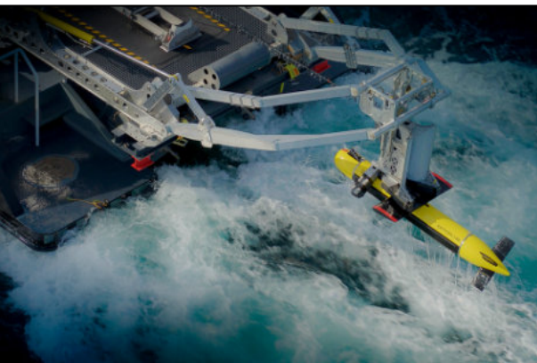
Katfish lowered from an A Frame
