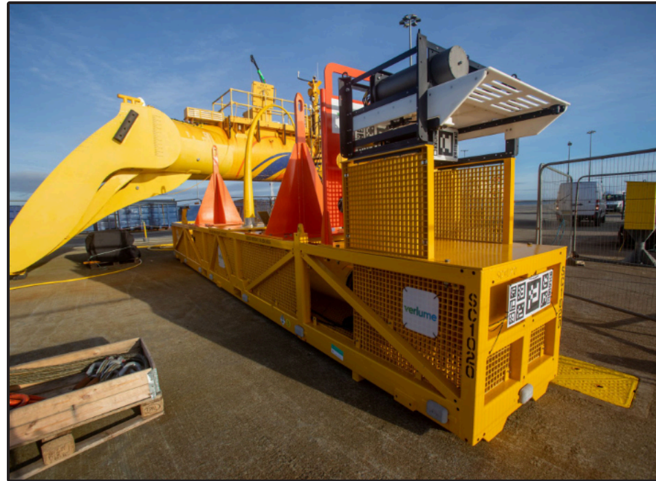
Subsea battery energy storage system and wave energy converter ahead of at-sea trials
