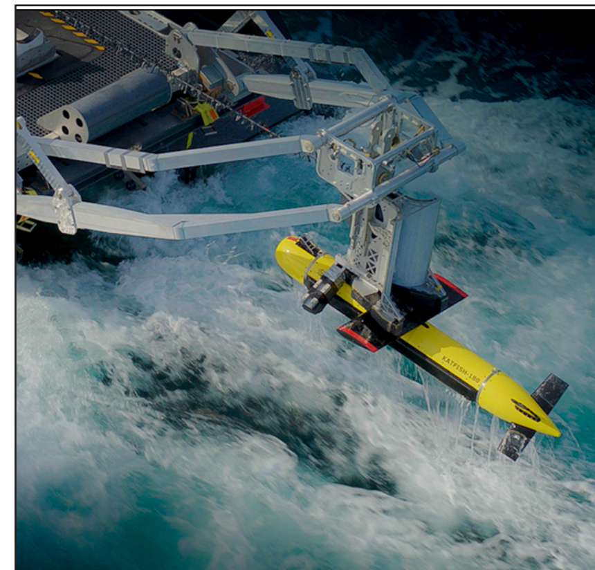
Katfish lowered from an A Frame
