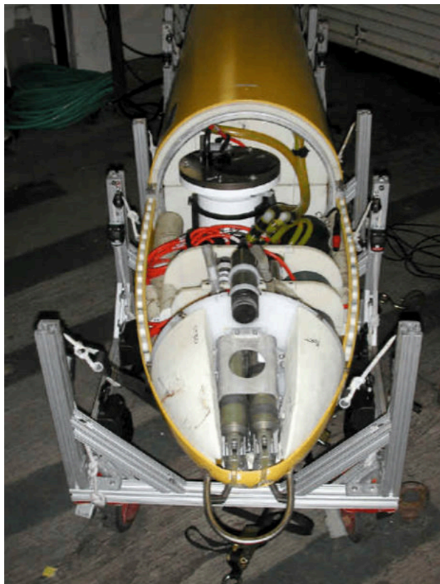
The nose of a Dorado with its outer "skin" removed, showing oceanographic sensors housed inside. Image: MBARI
