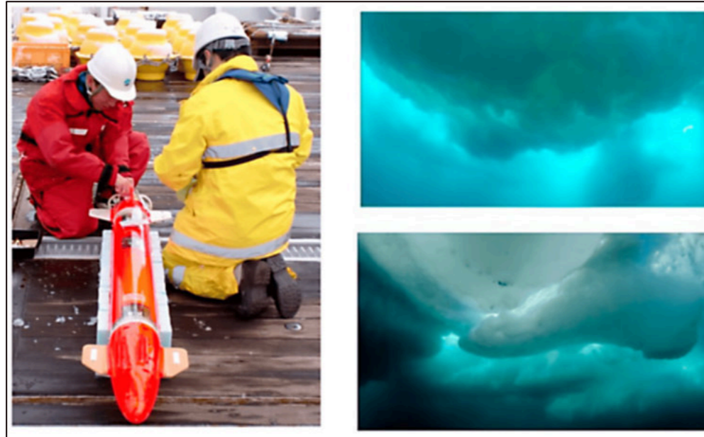
RAIV AUV and the images taken below sea ice (used with permission from JAMSTEC).
