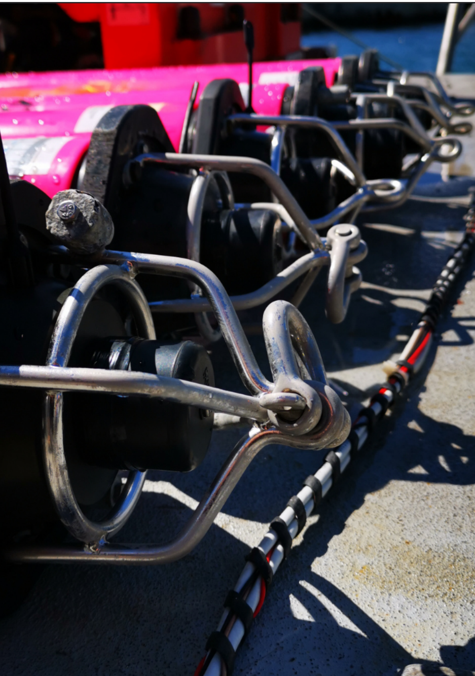
Canopus transponders being deployed during a positioning operation off the coast of Africa.
