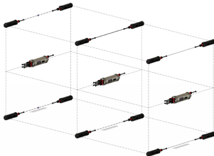
Hypermag Gradiometer arrangement
