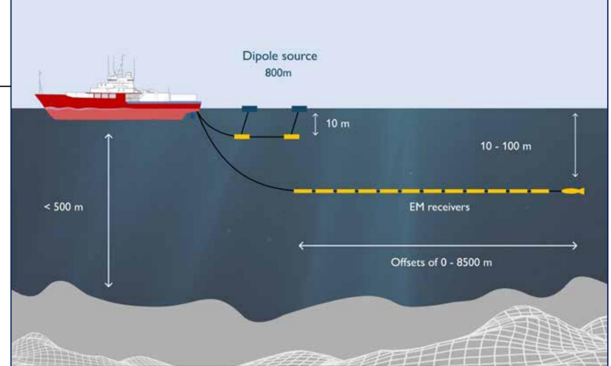
typically with a peak output current of 1.25kA, although source currents up to 7kA have been used.
