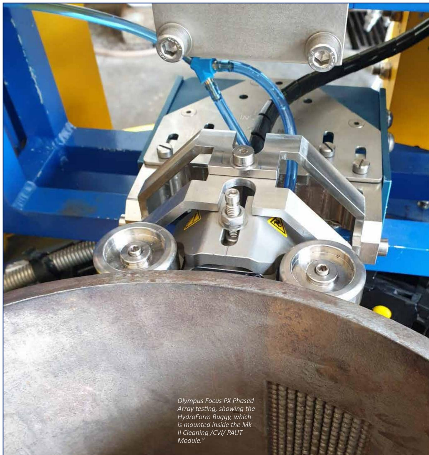
*Olympus Focus PX Phased Array testing, showing the HydroForm Buggy, which is mounted inside the Mk II Cleaning /CVI/ PAUT Module.”*
