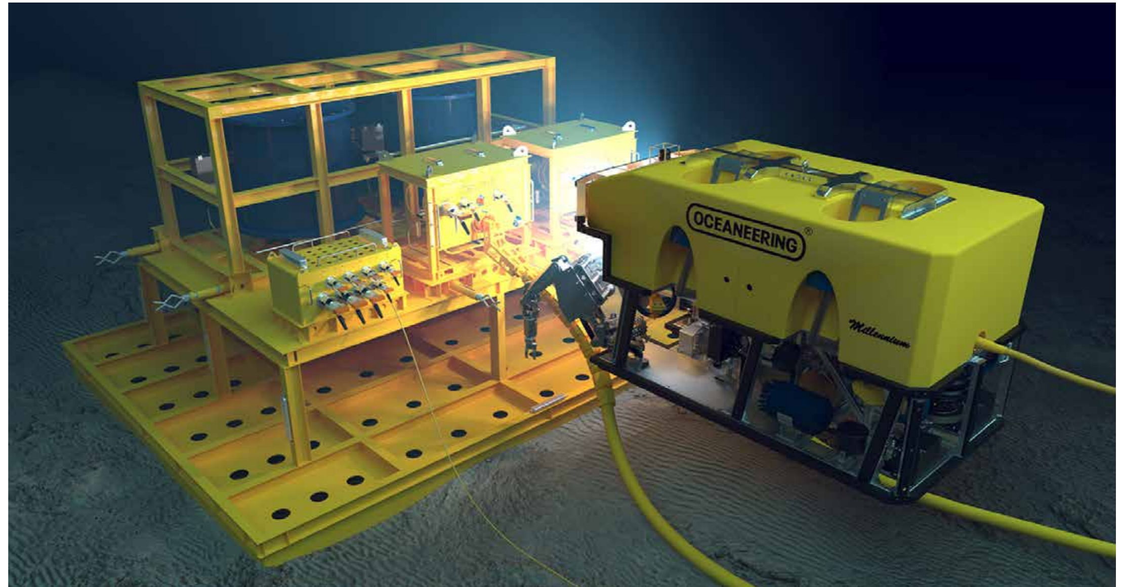
Subsea Pumping Technology unit with an Oceaneering ROV subsea.
