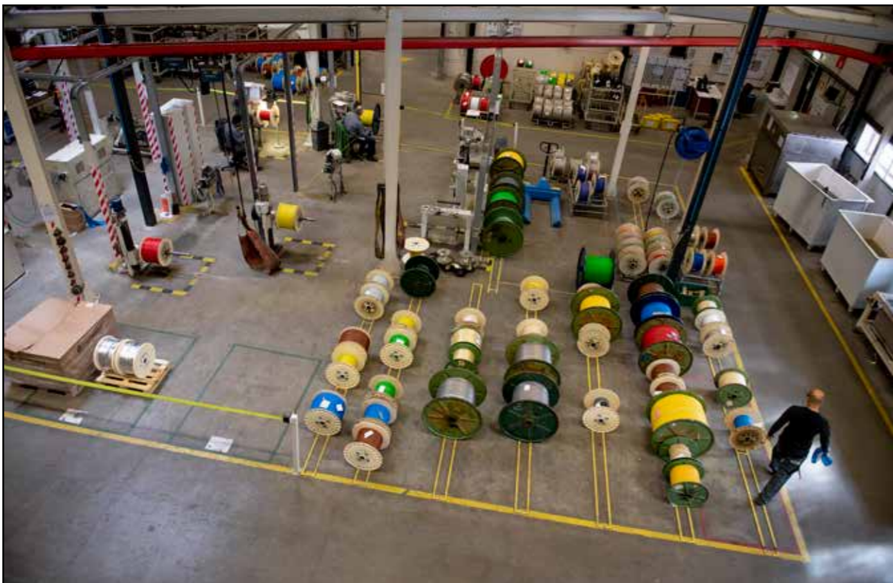
Stored bobbins containing individual cable subcomponents waiting to be installed on the lay up machine
